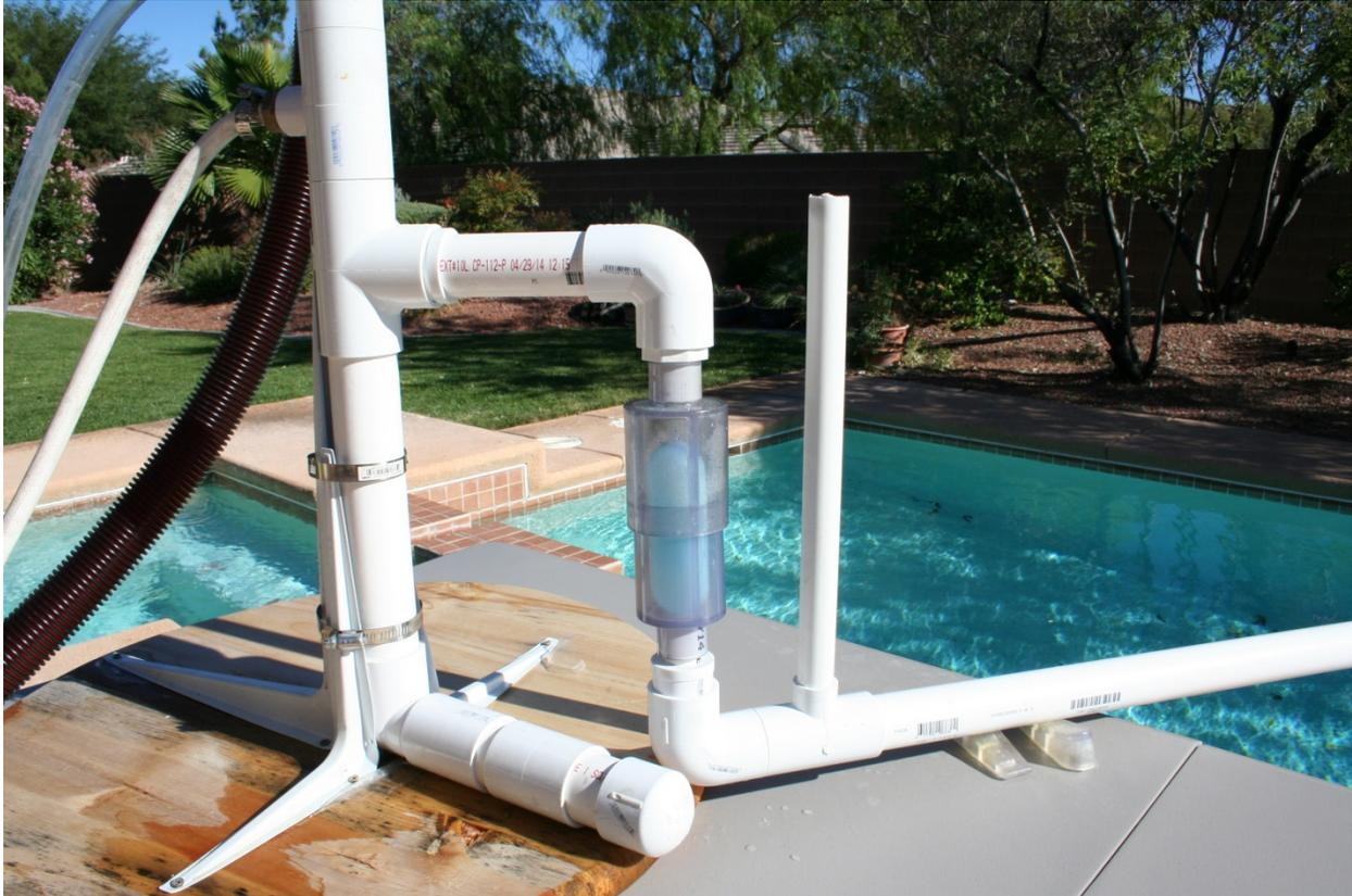
Figure 6. Positive Pressure P-Series HVAC **Air-Trap**<sup>®</sup> undergoing tests at the Des Champs Technologies Las Vegas, NV test facility. Testing videos showing the operation of the trap are viewable at [www.deschampstechnologies.com](http://www.deschampstechnologies.com), then go to P-Series and click on the link **P-Series YouTube Presentation**
