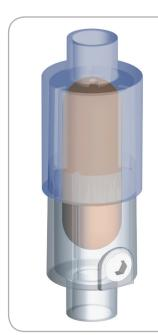
Des Champs Waterless Trap allows liquid condensate to drain from the HVAC equipment and simultaneously prevents air from entering or escaping from the equipment.
