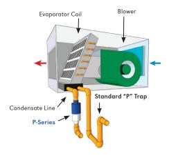
Note: The attached drawings represent traps that operate under positive pressure. Never connect condensate drain directly to a sanitary drain line.
